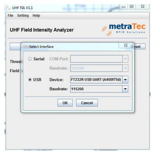
Select the  $\rightarrow$  Connect button and the software will connect to the sensor and display its ID and field strength in form of a column diagram. More columns are added in case more sensors are detected.
