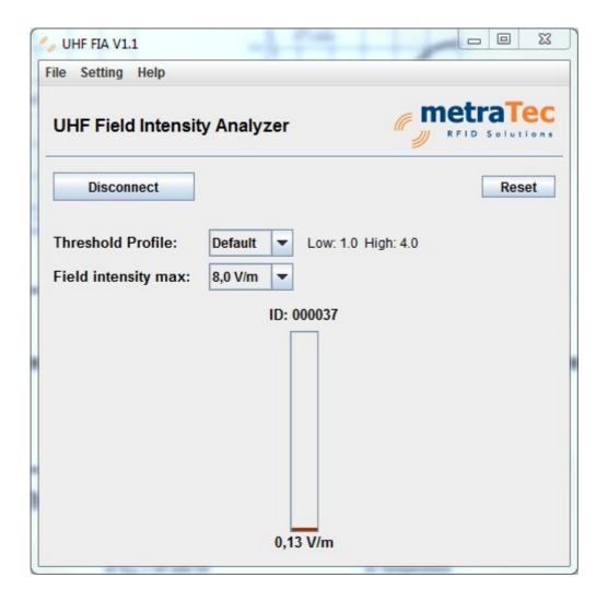
The → Reset button removes all connected sensors and resets the display to only the sensors that are still in range after the reset.
